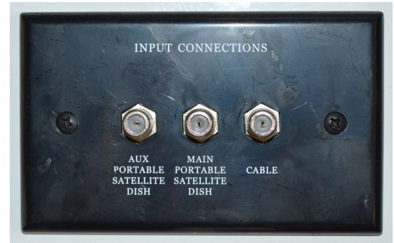
Satellite Dish and Cable TV Connections (Located in utility compartment, shoreline compartment, or water service center, depending on model) -Typical View
